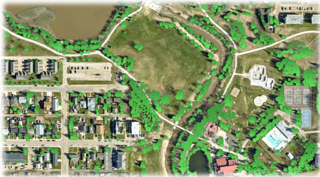
FIGURE 3 EXAMPLE OF LIDAR DETECTED AND DELINEATED TREE CROWNS USED TO MAP CANOPY CLOSURE IN MUSKOSEEPI PARK
