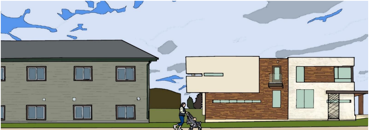
Figure 25 A Large Blank Façade on the Left in Contrast with the Design Guidelines Applied on the Right
