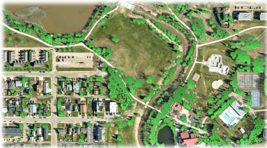
FIGURE 3 EXAMPLE OF LIDAR DETECTED AND DELINEATED TREE CROWNS USED TO MAP CANOPY CLOSURE IN MUSKOSSEPIE PARK
